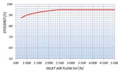
**Efficiency vs Air Inlet Air Flow:** This graph indicates the effect at inlet air flow variance on efficiency. Based on AC Coarse Test Dust with particle size ranging from sub-micronic to 200 microns, it illustrates the efficiency of the InoVane Tempest module through a wide range of inlet flows.
