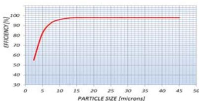
**Efficiency vs Particle size:** The InoVane Tempest has a dust removal efficiency of 98% for particles 15 microns and larger. This graph provides complete data on particle size removal efficiency showing that it will remove over 93% of all solid particles 8 micron or larger. In addition the InoVane Tempest has a water removal efficiency of over 90%.
