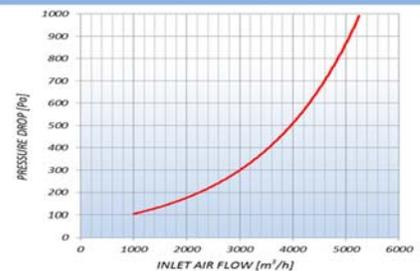
**Pressure Drop vs Air Inlet Air Flow:** Pressure drop through the InoVane Tempest is low (after the stationary spinners) due to the straight air path through the tubes. The graph shows a pressure drop of 270 Pa at an air flow of 2750 m³/h through the standard Tempest module.
